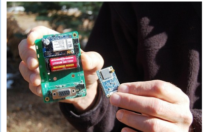
Low power computer components used in the snow depth wireless sensor network.
